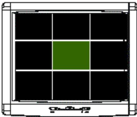
The green Area in the middle is the central area of the display with no more than one defective pixel.
